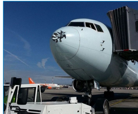
BIRDSTRIKE - 2013 / Geneva (Switzerland) - B767 Flight 830 Suffers Bird Strike During Landing
