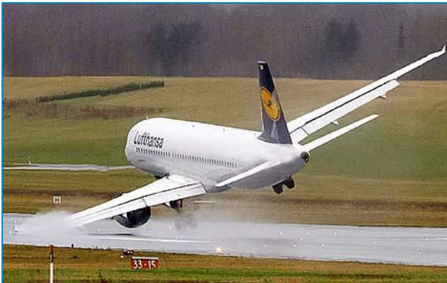
CROSSWIND - 2008/ Hamburg (Germany) –A320, wing touches runway in cross wind landing
