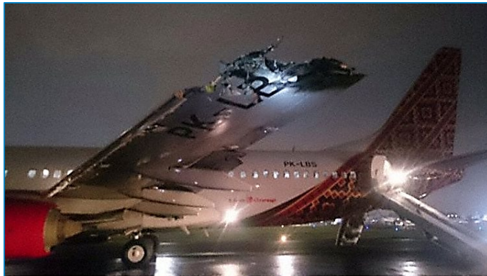
RWY COLLISION - 2016 / Jakarta (Indonesia) - B738 and AT42, collision on RWY, both aircraft on fire, TO clearance with towed aircraft on RWY
