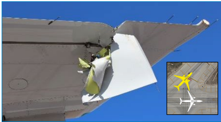
WINGTIP CLEARANCE – 2015 / Madrid (Spain) – B777 waiting for departure clearance at holding point. A330 taxiing , when overtake B777, struck between wingtips is produced.
